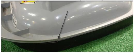
With the skirt (open side up) and hover mower sitting side-by-side on the ground, place the deck onto the skirt....
