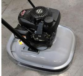
With the skirt in place, install the clamp brackets with 2 on the front, and 2 or 3 on the left and right side. NOTE: The deck and skirt may need to be pushed into place to fully seat together.
