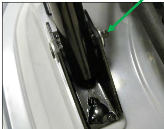
3. Attach the upper handle section to the lower handle section using the bolts and knobs. Fasten the corrugated tubing (which covers the throttle and engine stop cables) to the handles using the tie straps included.
