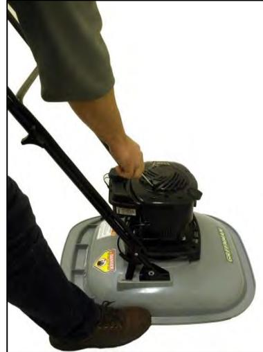
After the engine has started, carefully move behind the unit while continuing to grip the engine stop lever against the handle and adjusting your grip using both hands.
