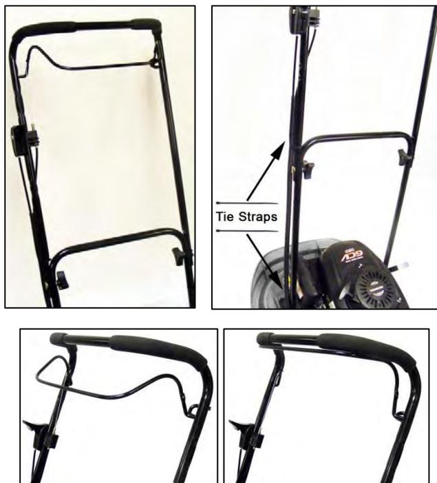
4. Verify that the engine stop lever is installed and it pivots upward completely against the handle.
