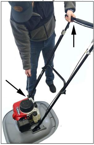
Pull the starter rope out slowly about 6-8" before beginning the full pulling motion and do not pull it all the way out. After the engine has started, move the choke lever to the OPEN position, then carefully move behind the unit while continuing to hold the stop lever against the handle and adjusting your grip position using **both** hands.
