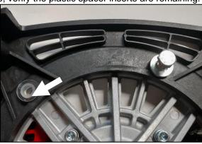
Place the mounting base onto the underside of the new engine verifying that it's in the correct position with the triangle mark pointing to the top of the engine / front of mower.
