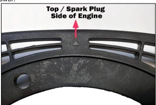
Insert bolts (with washers / spacers) then turn by hand to make sure they are threaded straight before tightening.
